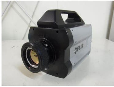
Fig.3 Infrared high-speed camera (FLIR X6900sc)
